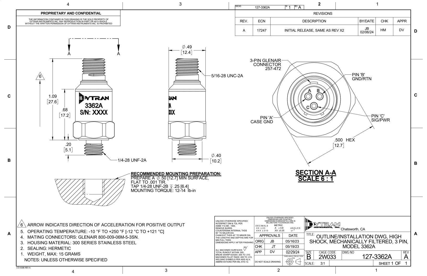
**Model Number** DOC NO PERFORMANCE SPECIFICATION 3362A PS3362A SHOCK ACCELEROMETER, IEPE REV A, ECN 17247, 02/06/24
